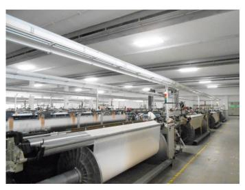
efficient equipment and reducing the electric load to a gigantic level Kohinoor now have added 48 looms more along with HVAC and other weaving shed items but the total power consumption is lowered to 4.5 Megawatt. This amazing saving has been achieved by making the new weaving shed most energy efficient.
